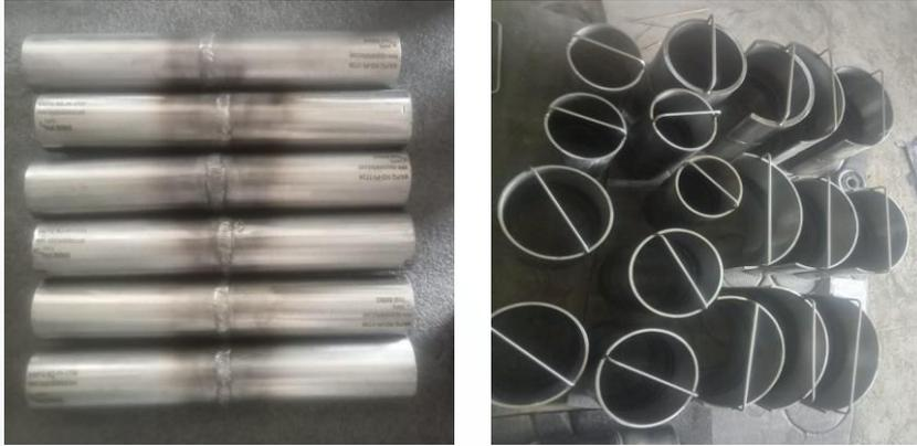
Our **NDT Flawed Specimens** are meticulously designed to replicate real-world defects, providing essential tools for training, evaluation, and validation of inspection techniques. These specimens enable NDT professionals to enhance their skills and ensure the accuracy of their testing processes in various NDT methods. This specimens available in various standards like **ASME, API, AWS, ISO 9712, SNT-TC-1A**
